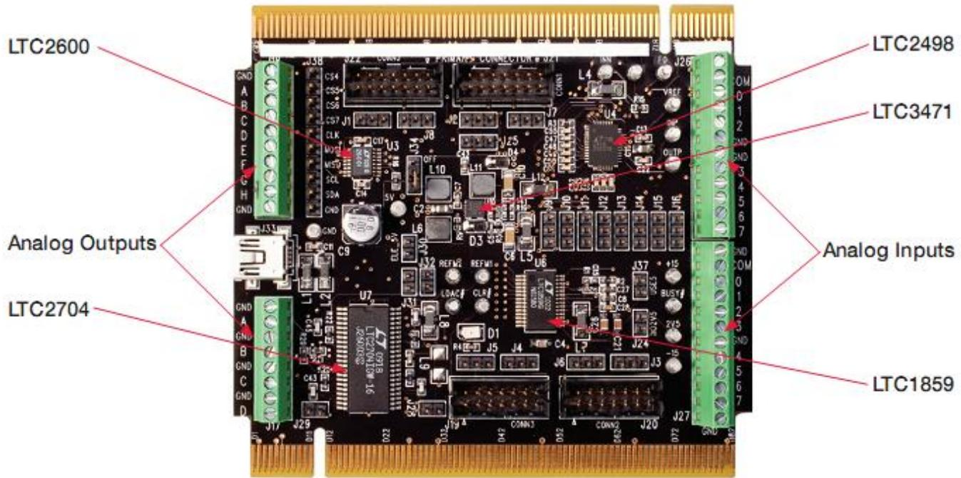
Figure 2. Callouts on top side of the TWR-ADCDAC-LTC
