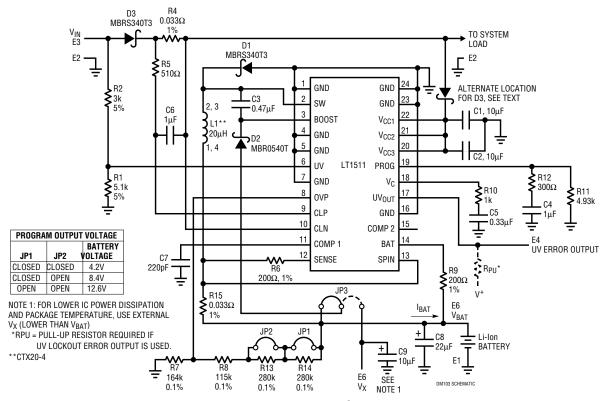
Figure 1. Demo Board Schematic
