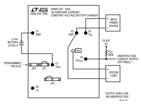
Figure 2. Typical Wiring Diagram of Demo Board
