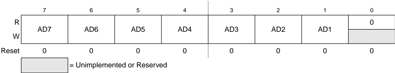
Figure 10-3. IIC Address Register (IICA)
