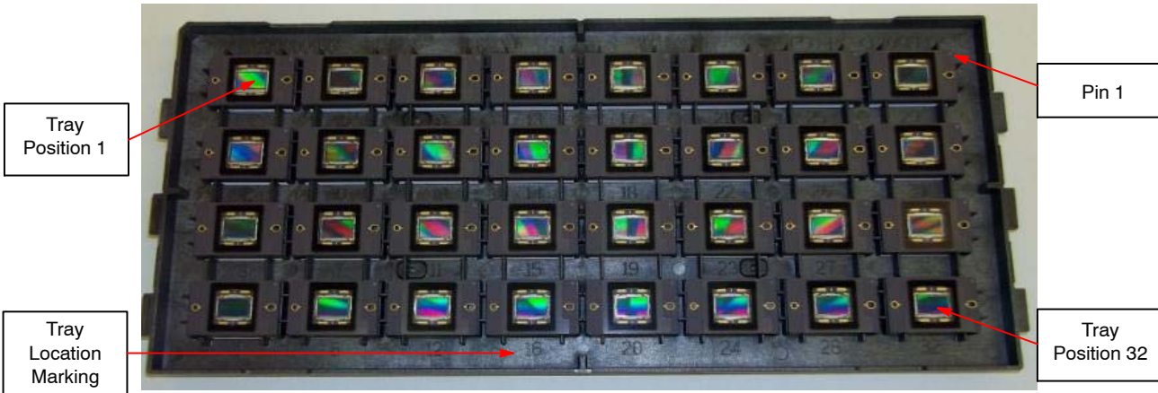
Figure 35. Tray Pin-Down View
