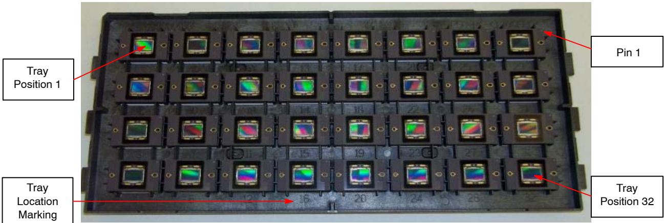
Figure 35. Tray Pin-Down View
