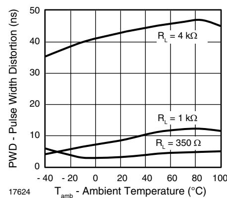
Fig. 16 - Pulse Width Distortion vs. Ambient Temperature
