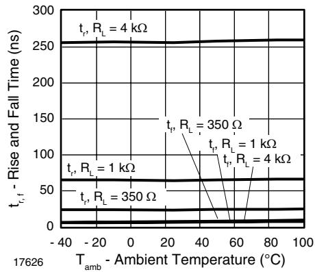
Fig. 18 - Rise and Fall Time vs. Ambient Temperature
