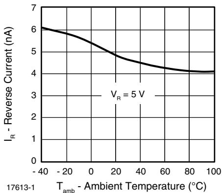
Fig. 5 - Reverse Current vs. Ambient Temperature
