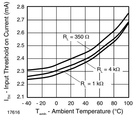
Fig. 8 - Input Threshold on Current vs. Ambient Temperature
