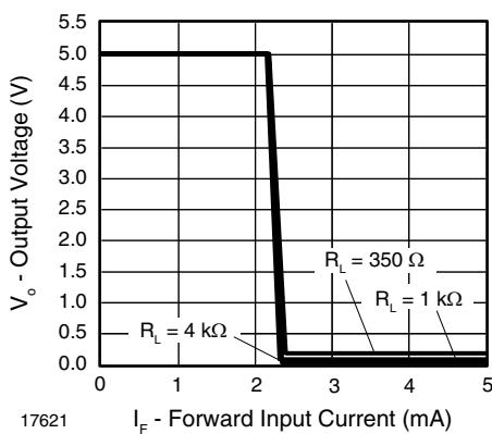
Fig. 13 - Output Voltage vs. Forward Input Current
