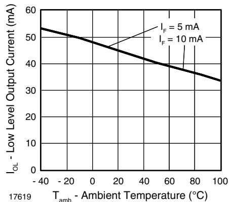
Fig. 11 - Low Level Output Current vs. Ambient Temperature
