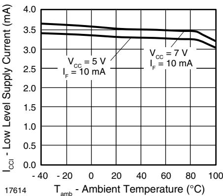
Fig. 6 - Low Level Supply Current vs. Ambient Temperature
