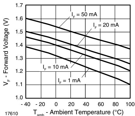
Fig. 3 - Forward Voltage vs. Ambient Temperature
