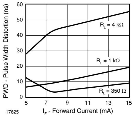
Fig. 17 - Pulse Width Distortion vs. Forward Current
