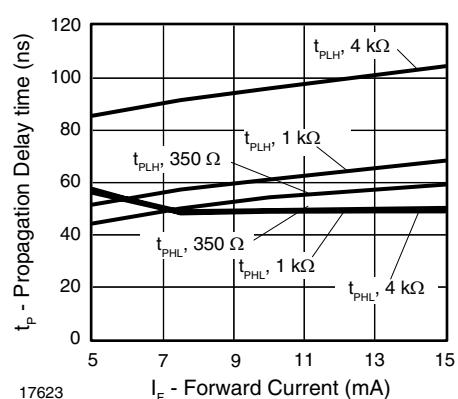
Fig. 15 - Propagation Delay vs. Forward Current
