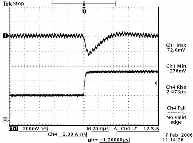
50% to 100% load Transient at 5.0 Vdc output
