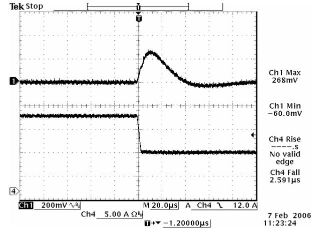
100% to 50% load Transient at 0.75 Vdc output
