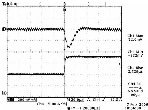
50% to 100% load Transient at 3.3 Vdc output
