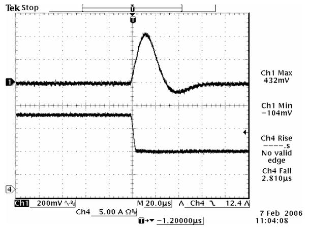
100% to 50% load Transient at 0.75 Vdc output
