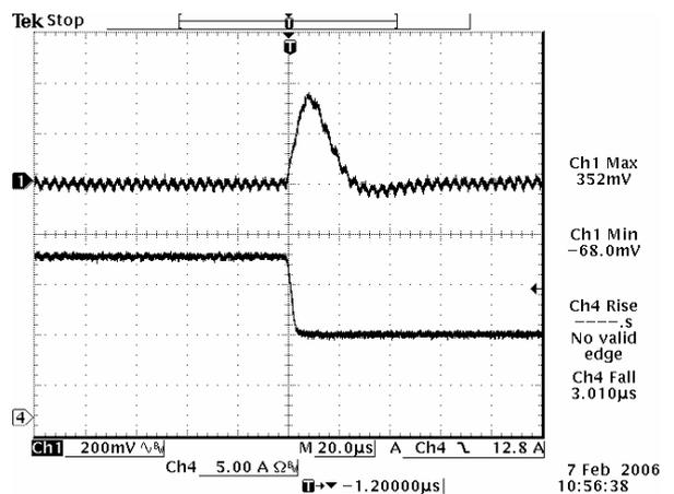
100% to 50% load Transient at 3.3 Vdc output
