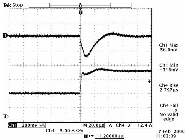
50% to 100% load Transient 0.75 Vdc output
