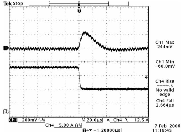
100% to 50% load Transient at 3.3 Vdc output
