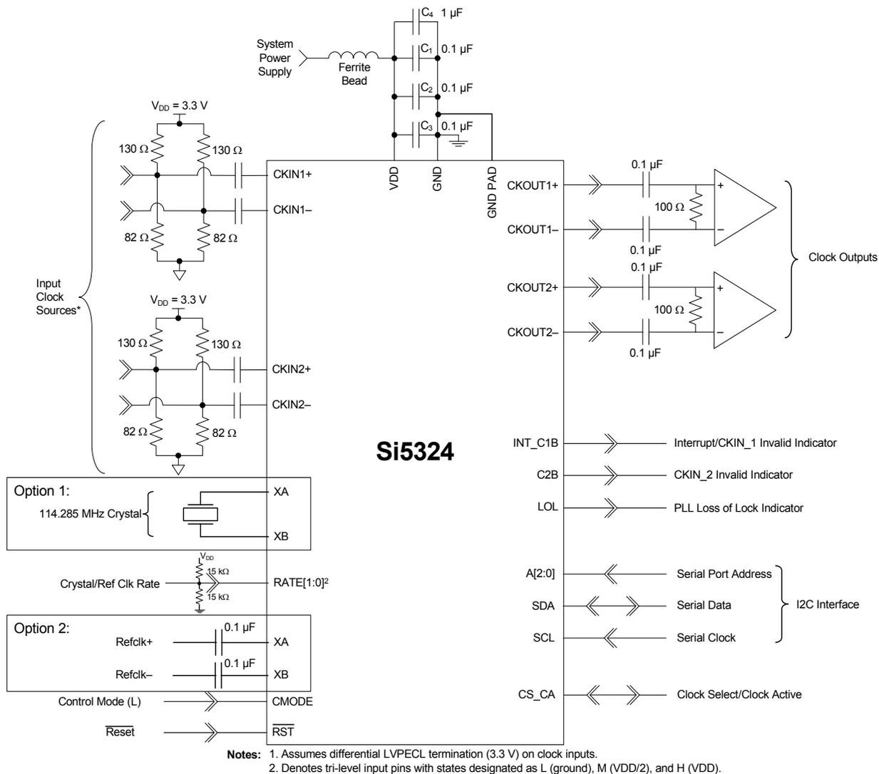
Figure 3. Si5324 Typical Application Circuit (I<sup>2</sup>C Control Mode)
