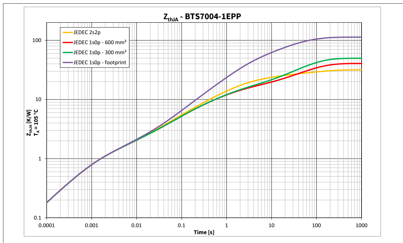
Figure 9 Typical Thermal Impedance. PCB setup according Chapter 4.4.1
