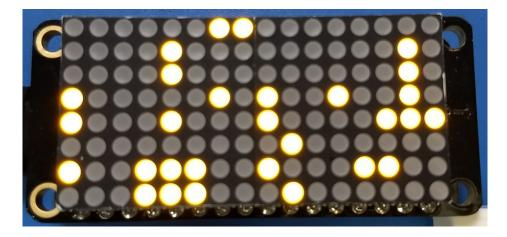
The above command will create the matrix class using the default I2C address of the display (0x70). If you've changed the I2C address (like when using multiple backpacks or displays) you can override it in the initializer using an optional **address** keyword argument.
