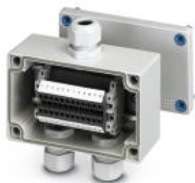
Terminal box, With 12 terminal blocks, 2.5 mm 2 with screw connection technology, material: ABS, gray, 130 mm x 80 mm x 60 mm, type of locking: Screw-on cover
