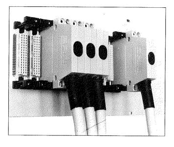
A particular advantage of this method of interconnection wiring is the wide variety of wiring methods that are possible. A female connector type chosen to suit the wiring method used (wire wrapping, solder, fast-on or piggy-back connections) is fitted in the interconnection field.
