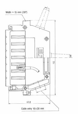
Cable housings KSG 203 for female connectors type F
