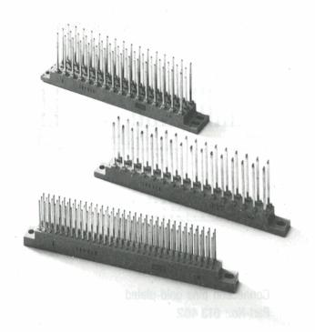
19" subracks have space for mounting female connectors to DIN 41 612 vertically in the wiring plane while the top and bottom edge wiring fields have room for mounting wiring strips and plug-on distribution strips horizontally. These strips are also suitable for mounting in the wiring plane. The wiring strips VE 64 and VE 96 with gold-plated 0,6 x 0,6 mm connection pins on a 2,54 mm grid are suitable for plugging on female connectors type C to DIN 41 612.
