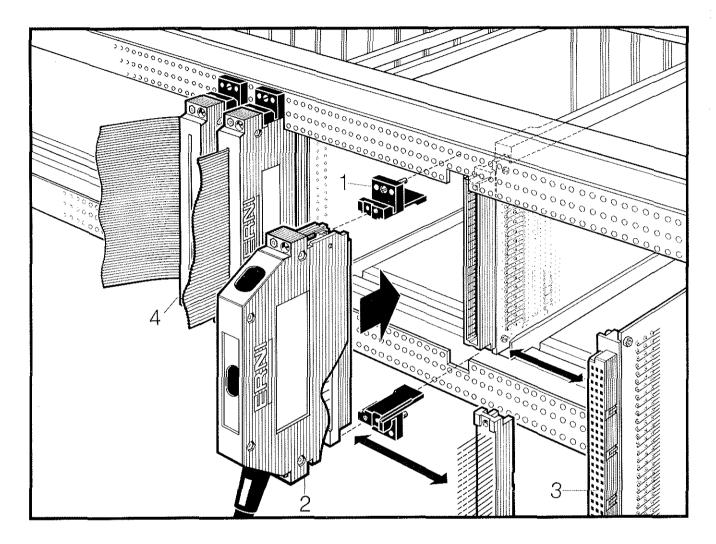
In a similar way to front-mounted connectors, this interface system also provides for making mateable interconnections directly from the wiring field to a printed circuit board. The guide elements are mounted on the rails of a subrack and serve to locate the PCB in the rack.
