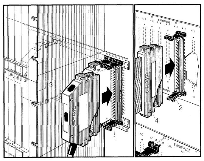
The interfacing technique shown in Pos. 1 is particularly suitable for cases and cabinets fitted with pivoting wiring frames.
