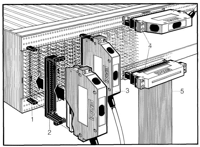
With this interface system, mateable interconnections can be provided on the wiring end between the internal wiring and the external wiring. Such connections can either be provided directly on the wiring plane or on the top or bottom edge fields.
