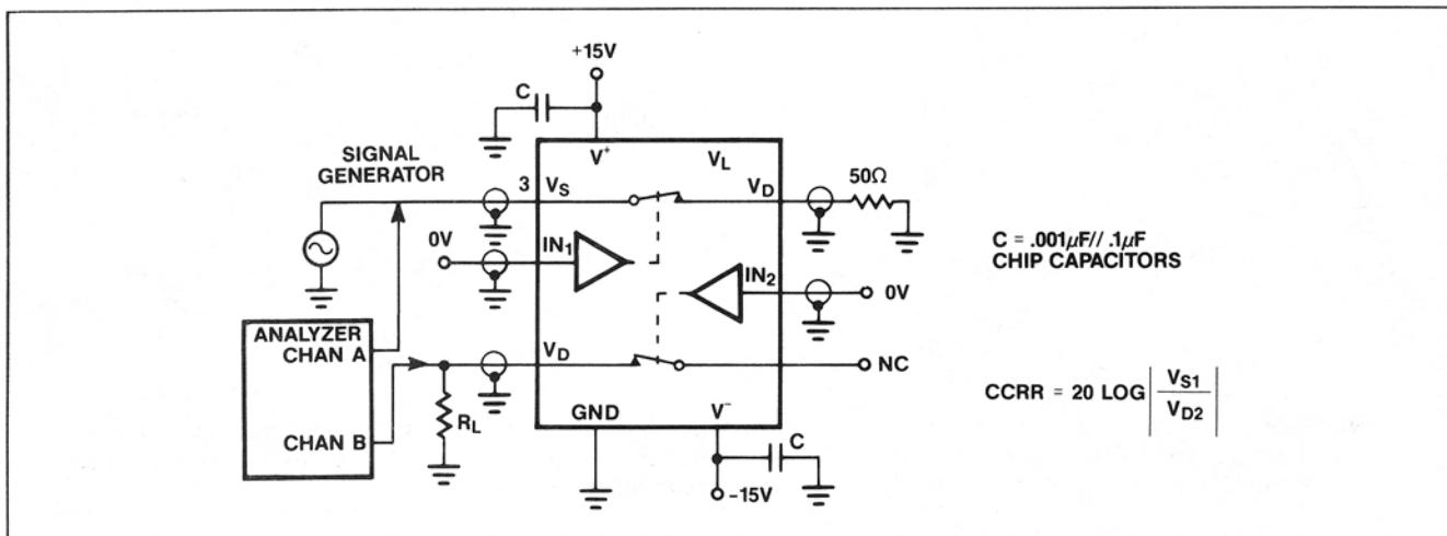
Figure 4. Channel To Channel Crosstalk Test Circuit
