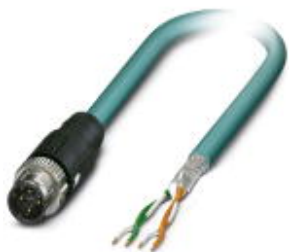
Network cable, Ethernet CAT5, 4-position, PUR, water blue RAL 5021, shielded, Plug straight M12 SPEEDCON / IP67, coding: D, on free cable end, cable length: 0.55 m
