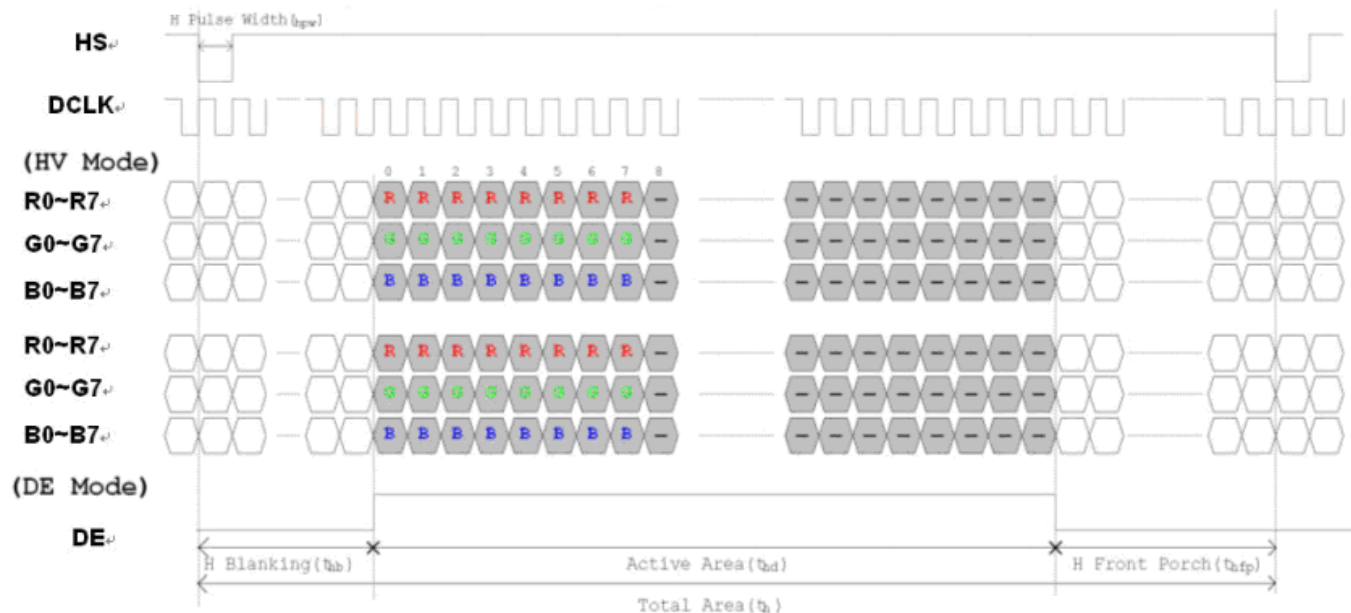
Figure 5: Horizontal Input Timing Diagram
