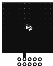
a. 65 ^{\circ}\text{C}/\text{W} when mounted on a 1 in 2 pad of 2 oz copper.
