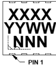
8-Lead DFN (3x3)(MCP662)
