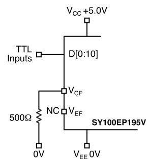
**Figure 9e. Connecting TTL Signals to the D Inputs, with V<sub>CC</sub> = 5.0V**
