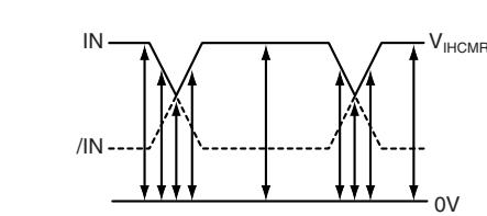
Figure 5a. Input Common Mode, PECL, LVPECL
