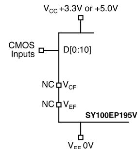
**Figure 9c. Connecting CMOS Signals to the D Inputs**
