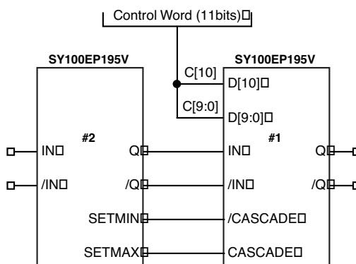
Figure 10a. Cascading Two SY100EP195V
