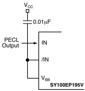
**Figure 7a. Interfacing to a Single-Ended PECL Signal**
