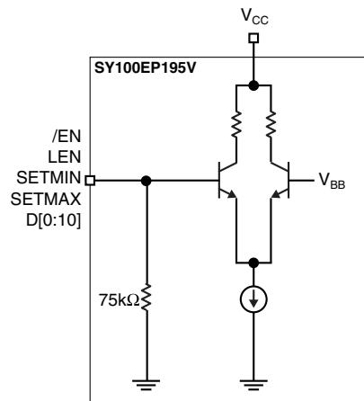
Figure 1b. Single-Ended Input Structure
