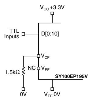
**Figure 9d. Connecting TTL Signals to the D Inputs, with V<sub>CC</sub> = 3.3V**
