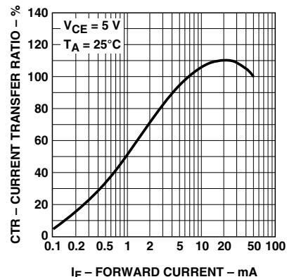
Figure 5. Current transfer ratio vs. forward current.
