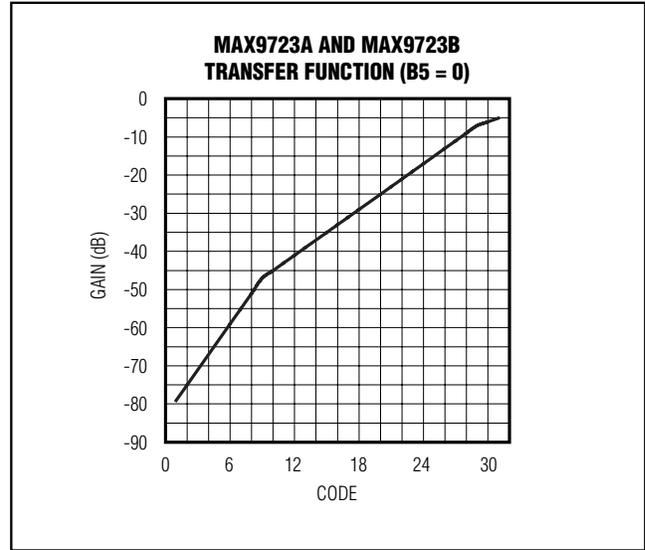
Figure 8. MAX9723A/MAX9723B Transfer Function with B5 = 0
