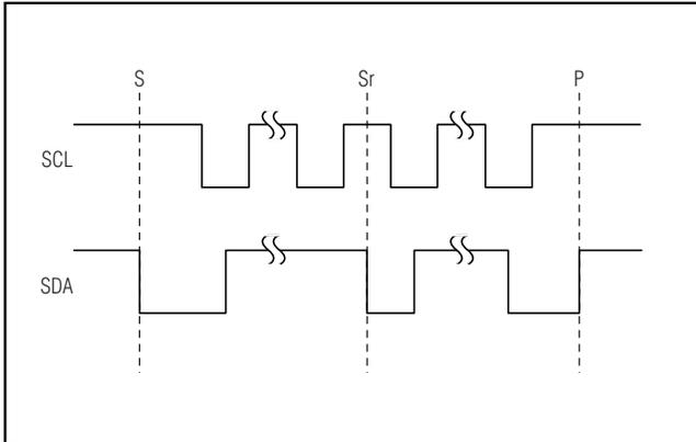
Figure 4. START, STOP, and REPEATED START Conditions
