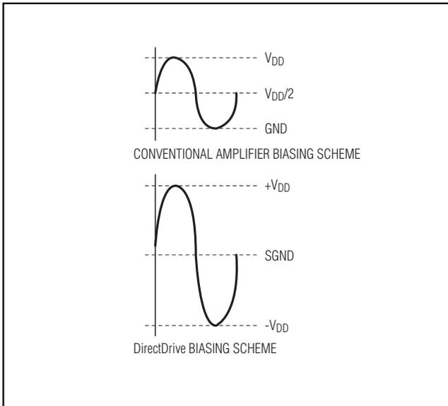
Figure 1. Traditional Amplifier Output vs. MAX9723 DirectDrive Output
