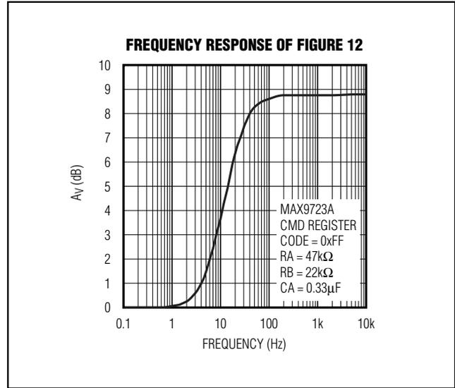
Figure 13. Increasing the Maximum Gain Using BassMax
