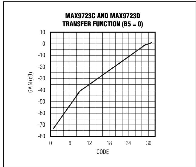
Figure 10. MAX9723C/MAX9723D Transfer Function with B5 = 0
