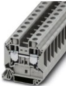
Feed-through terminal block, Connection method: Screw connection, Cross section: 1.5 mm 2 - 25 mm 2 , AWG: 16 - 4, Width: 12.2 mm, Height: 54.4 mm, Color: black, Mounting type: NS 35/7,5, NS 35/15
