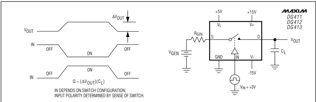
Figure 4. Charge-Injection
