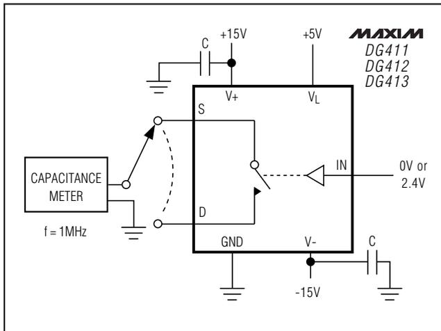
Figure 7. Channel Off-Capacitance
