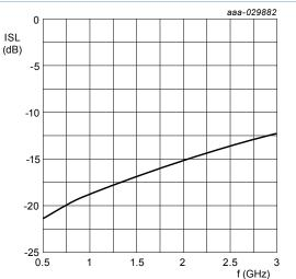
Diode zero biased and inserted in series with a 50  $\Omega$  strip line circuit. T<sub>amb</sub> = 25 °C.
