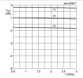
Diode inserted in series with a 50  $\Omega$  strip line circuit and biased via the analyzer T-network. T<sub>amb</sub> = 25 °C.
