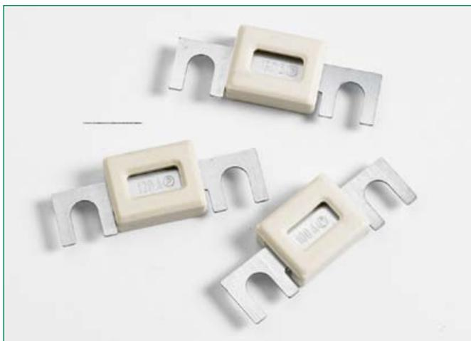
Housed fuse strips with window for visual inspection of melting element. Current rating 30A - 150A, 80 VDC. 90° fork type lugs.
