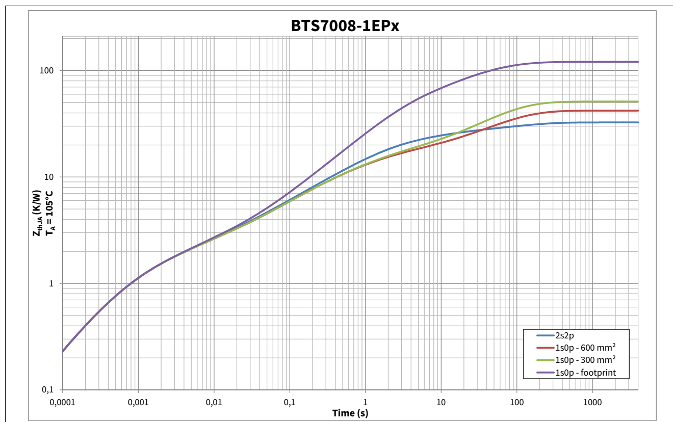
Figure 9 Typical Thermal Impedance. PCB setup according Chapter 4.4.1
