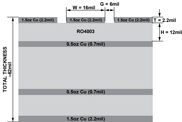
Figure 37. Evaluation Board Stackup
