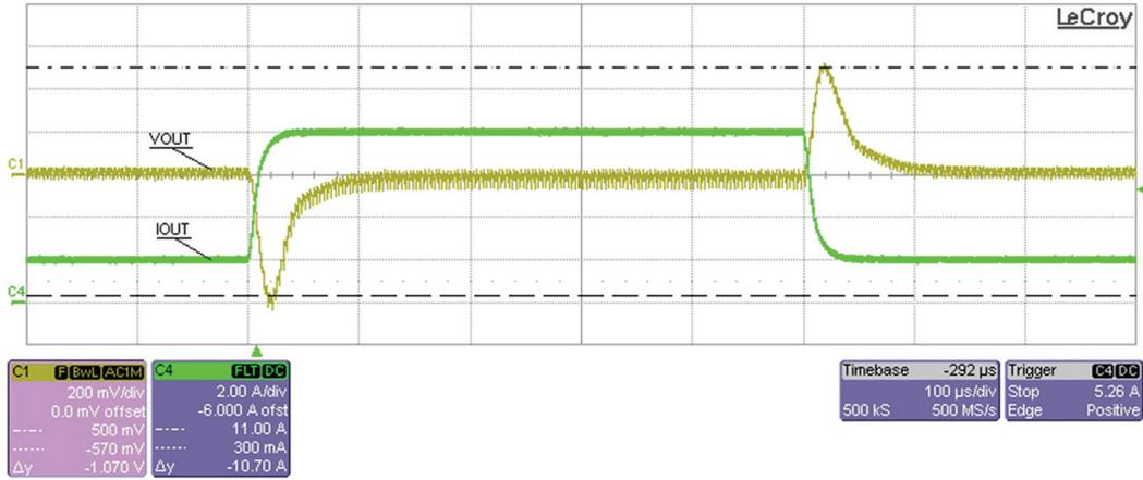
Figure 4. DC1619A 2A to 8A Load Transient
