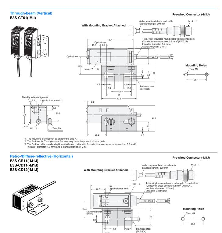
Note: Models numbers for Through-beam Sensors (E3S-CT61(-M1J)) are for sets that include both the Emitter and Receiver.
