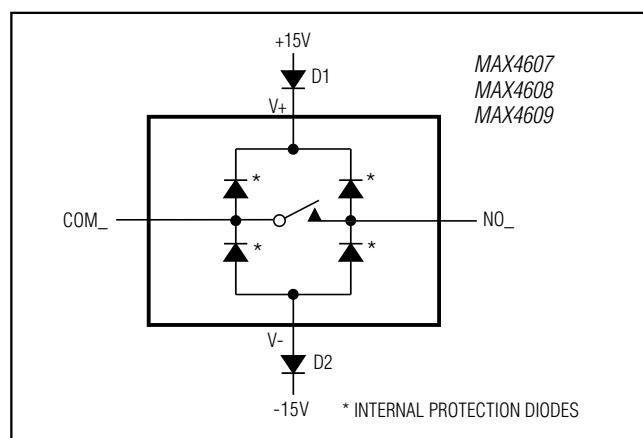
Figure 1. Overvoltage Protection Using External Blocking Diodes
