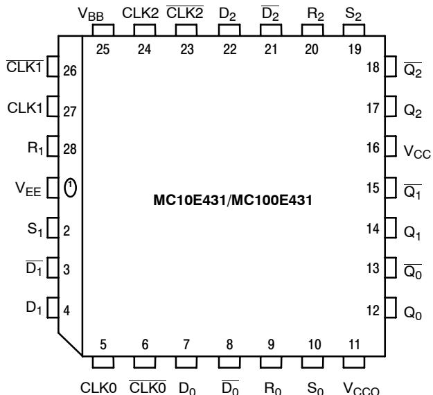
\* All V<sub>CC</sub> and V<sub>CCO</sub> pins are tied together on the die.
