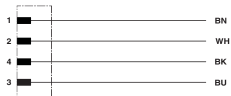
Contact assignment of the M8 plug
