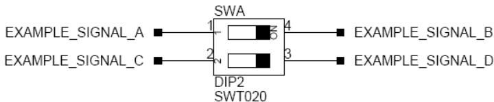
Figure 2-3. Example of Mechanical Switch Equivalent to [Figure 2-2](#)
