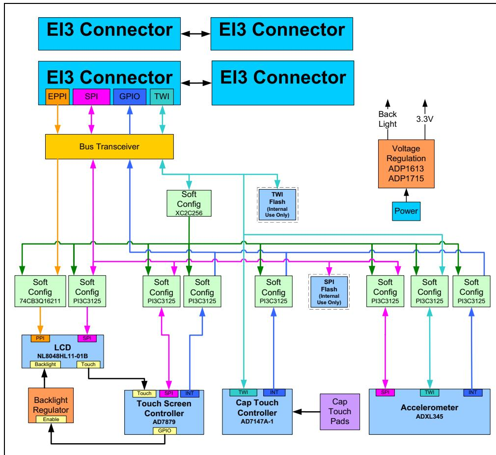
Figure 2-1. Block Diagram
