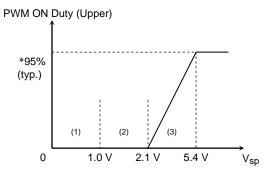
\*: The maximum ON duty is  $T_{on} = 95\%$  (typ.) when  $V_{SP} = 5.4 \text{ V}$  (typ.).
