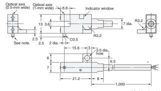
$^{\star}$  Vinyl-insulated round cable of 3.5 dia., 3 cores, (0.14 mm² with 1.0-dia. insulator); Standard length: 1 m  $\,$
