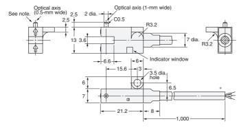
\* Vinyl-insulated round cable of 3.5 dia., 3 cores, (0.14 mm² with 1.0-dia. insulator); Standard length: 1 m
