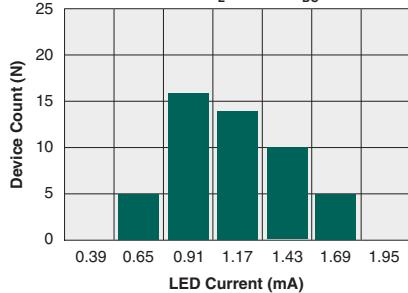
**Typical  $I_F$  for Switch Dropout
