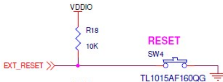
Figure 10. Using EXT_RESET pin
