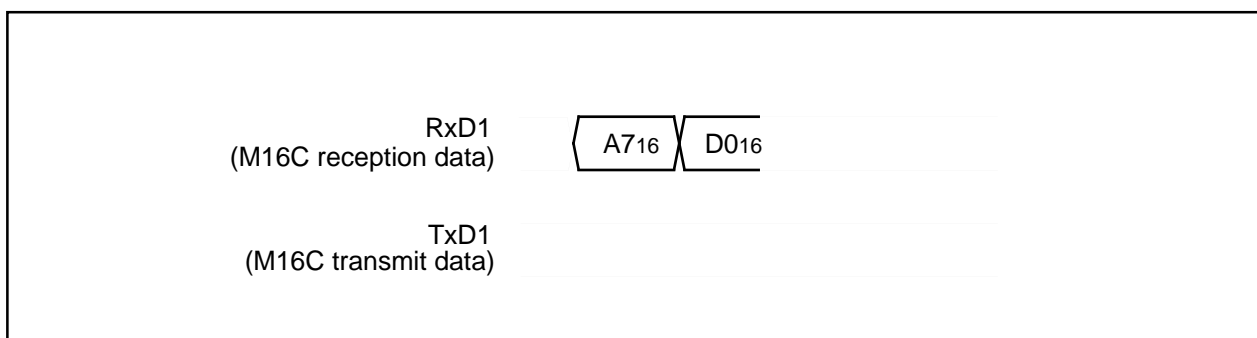
Figure 1.29.28. Timing for erasing all unlocked blocks
