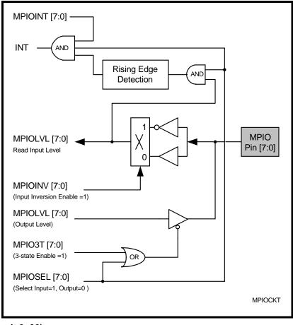
FIGURE 8. MULTIPURPOSE INPUT/OUTPUT INTERNAL CIRCUIT
