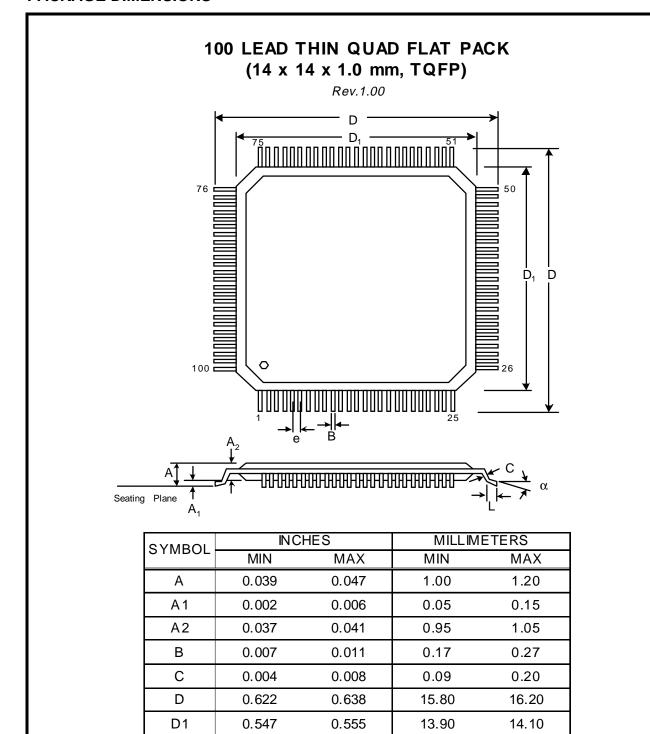
Note: The control dimension is in millimeter.
