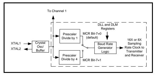
Programming the Baud Rate Generator Registers DLM and DLL provides the capability for selecting the operating data rate. Table 9 shows the standard data rates available with a 14.7456 MHz crystal or external clock at 16X clock rate. At 8X sampling rate, these data rates would double. When using a non-standard data rate crystal or external clock, the divisor value can be calculated with the following equation(s).
