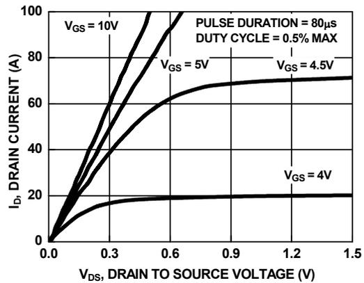
Figure 8. Saturation Characteristics
