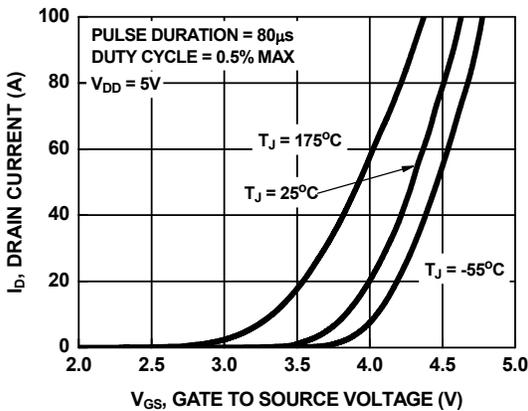
Figure 7. Transfer Characteristics
