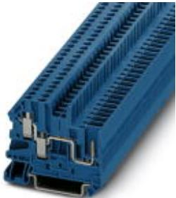
Feed-through terminal block, Connection method: Screw/plug-in connection, Cross section: 0.14 mm<sup>2</sup> - 4 mm<sup>2</sup>, AWG: 26 - 12, Width: 5.2 mm, Color: blue, Mounting type: NS 35/7,5, NS 35/15
