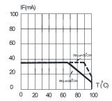
FIG.5 Blue MAXIMUM FORWARD DC CURRENT VS AVBIENT TEMPERATURE (Tjmax=110 $^{\circ}$ C)
