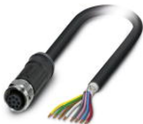
Sensor/Actuator cable, 8-position, PE-X/PE-X halogen-free, black-gray RAL 7021, shielded, free cable end, on Socket straight M12, A-coded, Cable length: 10 m, for outdoor applications, with high-grade steel knurl
