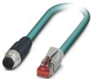
Assembled Ethernet cable, shielded, 4-pair, 26 AWG stranded (7-wire), RAL 5021 (water blue), M12 plug to RJ45 plug/IP20, line, length 10 m
