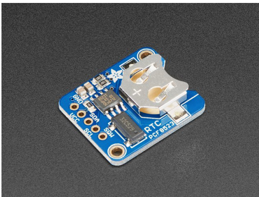
Adafruit PCF8523 Real Time Clock Assembled Breakout Board
