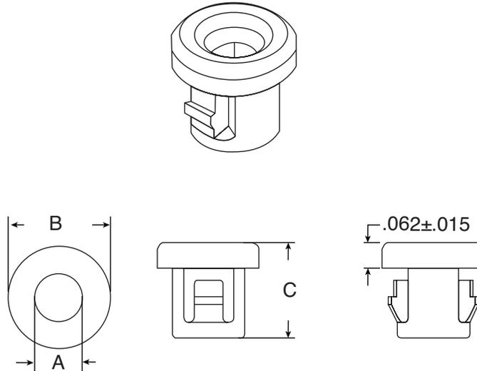
Bushings provide economical protection for wire, cable, tubing, and hose from sharp, uneven drilled or punched holes in sheet metal.
