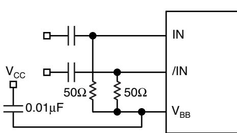
**Figure 13. Re-Biasing an AC-Coupled Signal**
