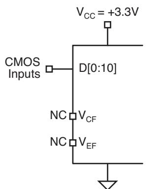
**Figure 12.  $V_{CF}/V_{EF}$  Biasing for CMOS Control (D) Input**
