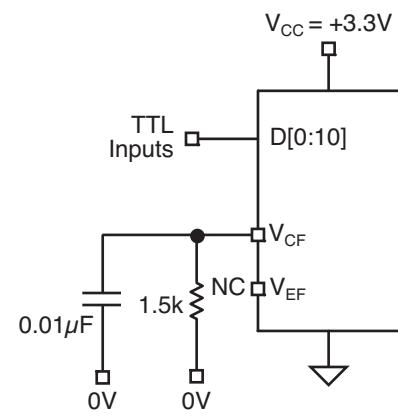
**Figure 14.  $V_{CF}/V_{EF}$  Biasing for LVTTL Control (D) Input**
