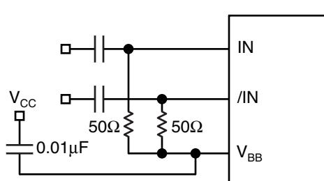
**Figure 13. Re-Biasing an AC-Coupled Signal**
