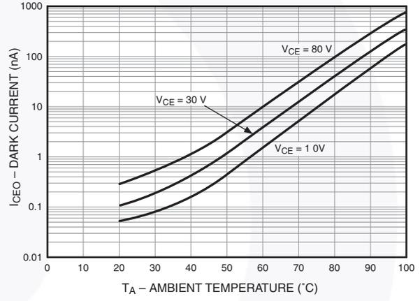
Figure 6. Collector-Emitter Dark Current vs. Ambient Temperature
