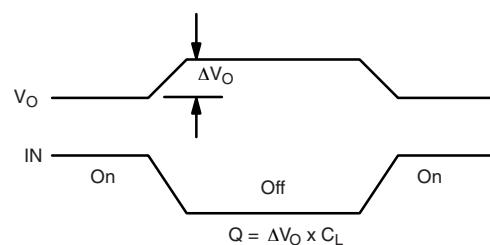
Figure 4. Charge Injection
