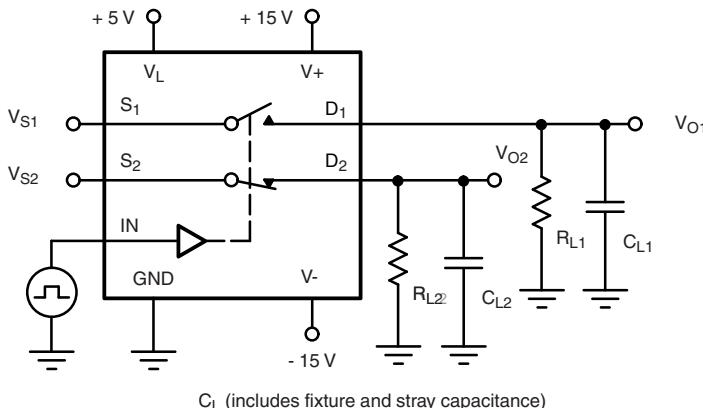
$C_L$  (includes fixture and stray capacitance)
