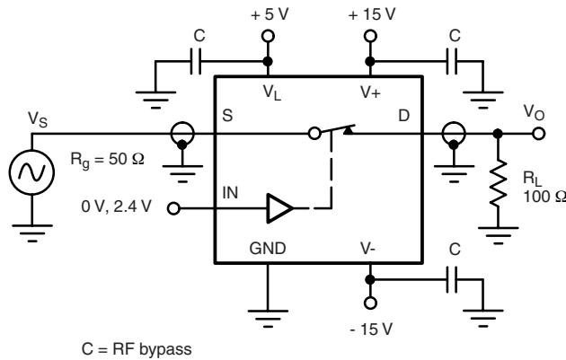
**Figure 6. Insertion Loss**
