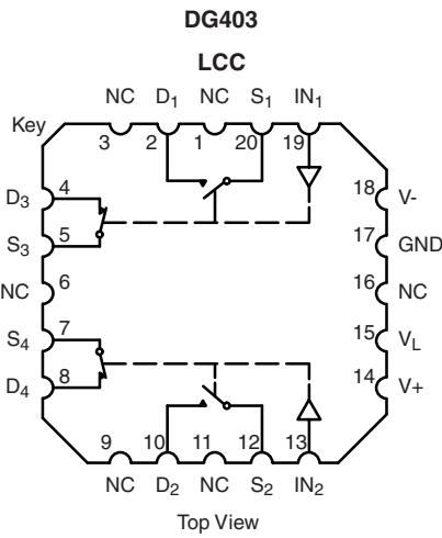
Two SPDT Switches per Package
