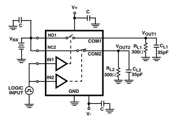
C<sub>L</sub> includes fixture and stray capacitance. Reconfigure accordingly to test SW3 and SW4.
