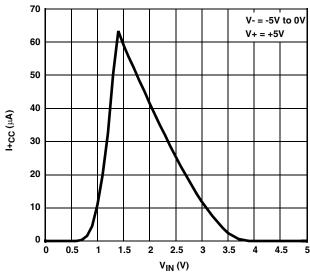
FIGURE 18. POSITIVE SUPPLY CURRENT vs DIGITAL INPUT VOLTAGE
