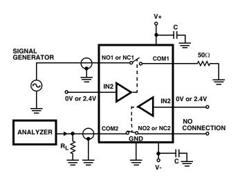
FIGURE 6. CROSSTALK TEST CIRCUIT
