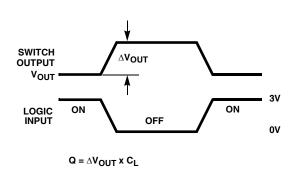
Logic input waveform is inverted for switches that have the opposite logic sense.
